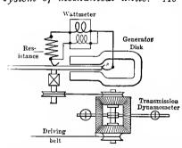
FIG. 23. Diagram showing generator disk driven through differential transmission dynamometer to measure mechanical power input.
